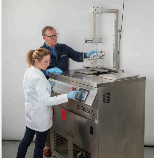
Fluid extraction of the binders can be easily done with a vapor degreaser.
