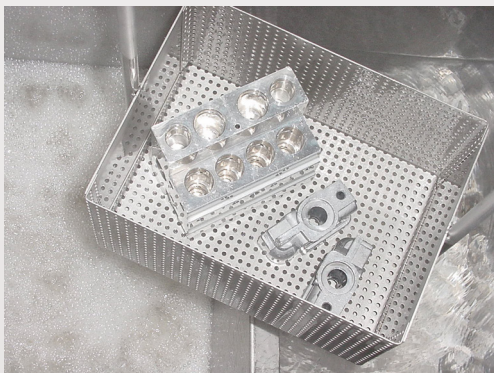
Debinding may be performed in either the vapor or liquid phase in the vapor degreaser.
